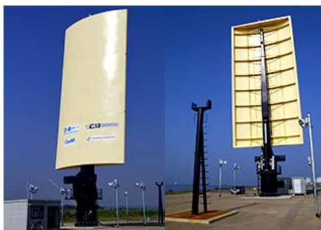
Photo 1: Power Assist Sail prototype
